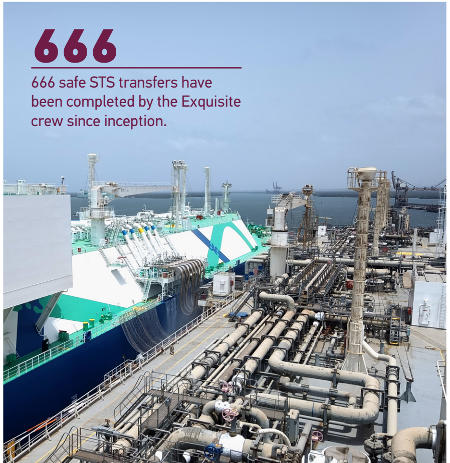
Nakilat vessel FSRU 'Exquisite' plays a vital role in converting LNG into natural gas for Pakistan's national grid.
